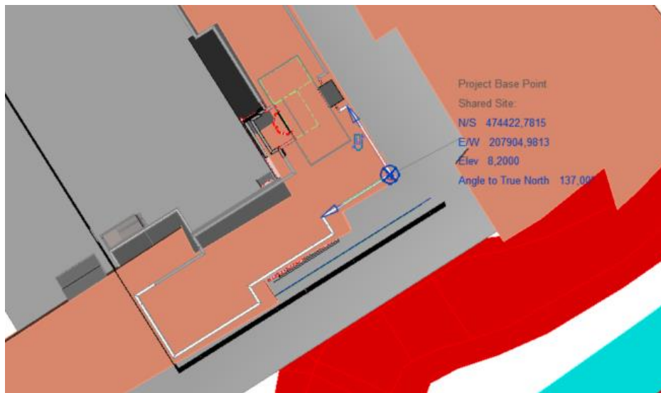
Figure 8- Sharing the coordinate system of layers from Civil3D to Revit
