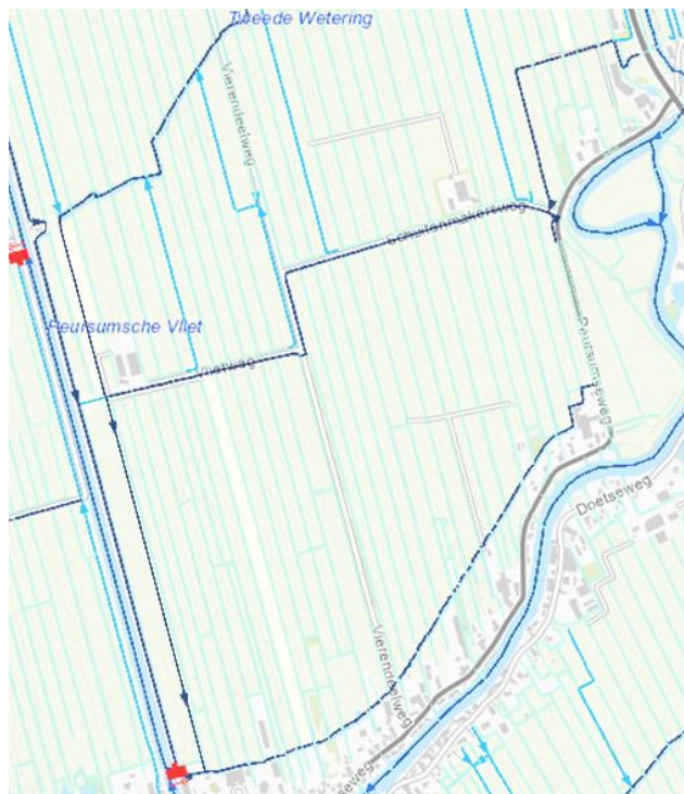
Figure 22: Closer look at water flow in scenario 2 bridging period; in the bridging period some connection between the new and the current channels are still in place
