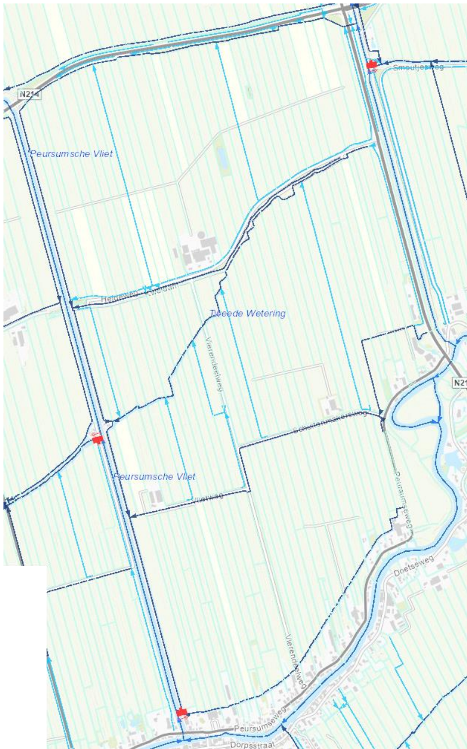
Figure 10: Waterflow in the area; Water is drained out the polder following the blue arrow in the figure which is approximately from north to south after east to west. The colour of blue depicts the magnitude of the channel, the darker blue are bigger drainage channels (among others the side channels of the Peursumse Vliet), the slightly lighter blue are smaller channels, and the light blue are small ditches. The water is drained of the polder via the pumping station in the southwest, depicted with a red icon.
