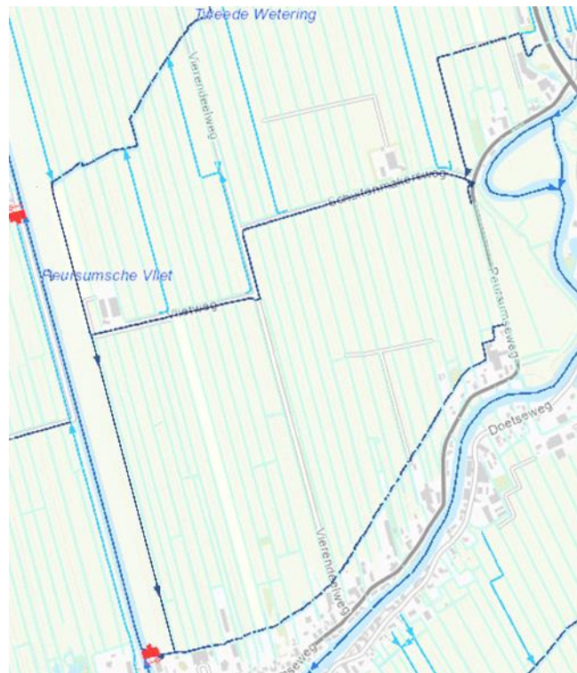
Figure 23: Closer look at water flow in scenario 2 after embankment reinforcement; the current channels is gone, and no connection are still present
