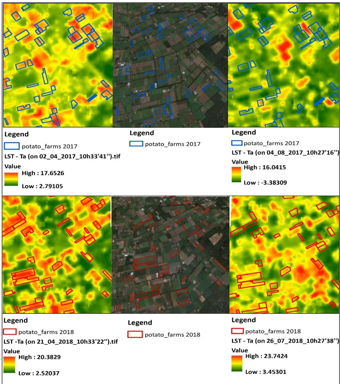
Figure 27: Comparison analysis of LST – T a or dT sa maps in two growing seasons, with middle google earth image for the real situation on the field during the study period.
