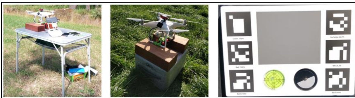
Figure 2-3: Sequoia camera mounted on DJI Phantom 4 Pro and AIRINOV target
