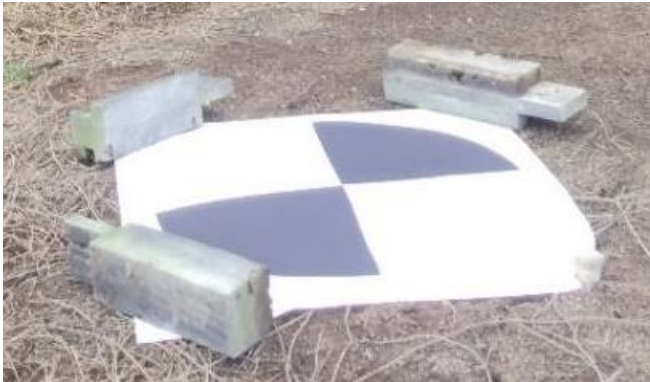
Figure 2-4: Recording 3-D coordinate of GCP with DGNS RTK in an open space
