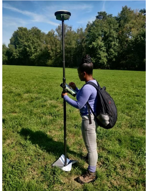
Figure 2-4: Recording 3-D coordinate of GCP with DGNS RTK in an open space
