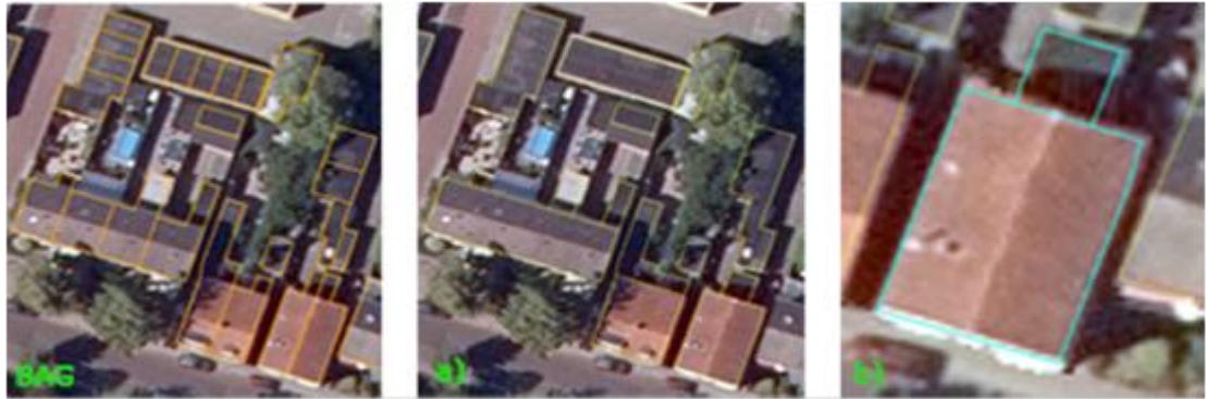
Figure 7-Modifications to BAG- a) Merging the buildings sharing the same roof, b) Splitting the flat and shaped parts
