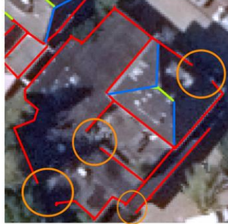
Figure 19- Failure of extending command to fix incomplete lines
