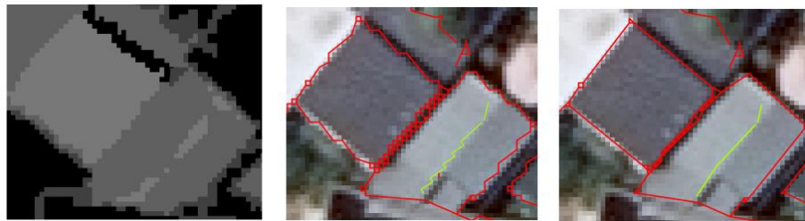
Figure 17- The prediction artefacts- left nDSM, middle initial prediction without simplification, right simplified lines
