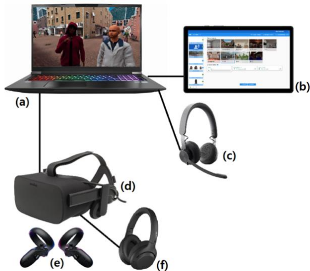
Figure 1. Setup of VR consisted of laptop (a), tablet with dashboard of “Triggers&Helpers” application (b), voice-morphing microphone (c), VR glasses (d), VR controllers (e), noise cancelling headphone (f).
