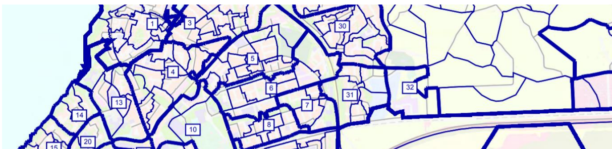
Figure 2.3: Zoning system of traffic model Harderwijk, zones (small blue lines) are based on aggregated PC6 regions and align with districts and quarters (thick blue lines) (Oranjewoud, 2009)
