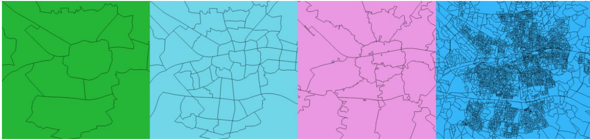
Figure 2.4: Different aggregation levels of CBS data in the city of Enschede, from left to right: districts, Quarters, PC4, PC6
