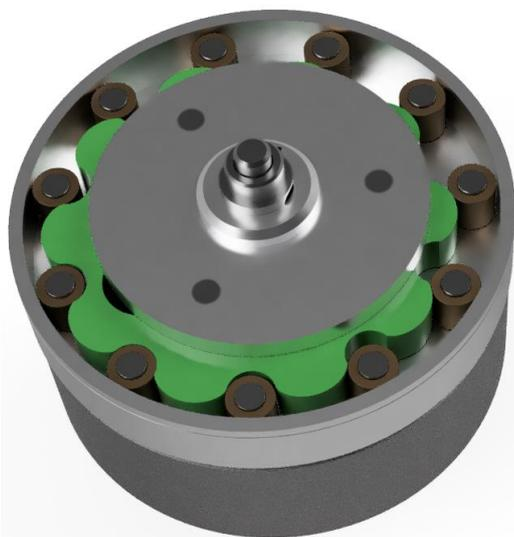
The new design features a novel cycloidal drive transmission that is designed to feature a larger gear ratio within a smaller space. While also providing a smooth power delivery and high load capability's
