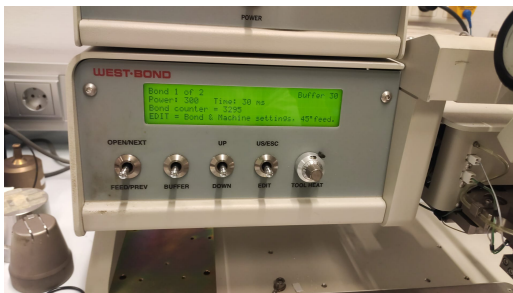
Figure 64: Wire bonder interface with buffer 30 selected
