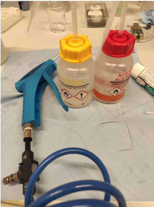
Figure 58: Aceton, Isopropanol 2 and the dry blower used to clean the PCB
