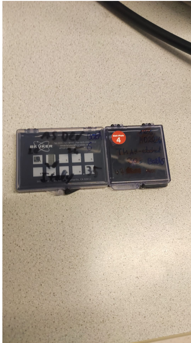
Figure 49: Special chip boxes/containers that contain an adhesive layer to stick the chips in
