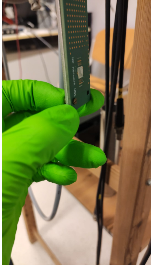
Figure 67: PCB attached to the dipstick and screwed in place with a nut
