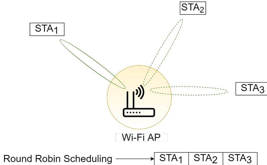
Figure 3.5: The representation of round robin scheduling used in WiFi-AP to transmit data towards its users.
