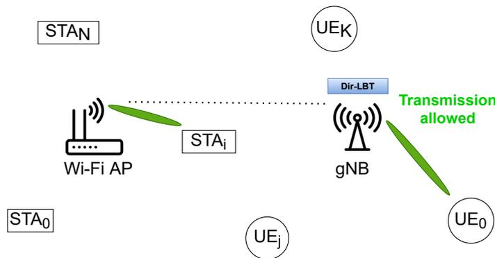
Figure 2.2: Dir-LBT senses along the transmission beam
