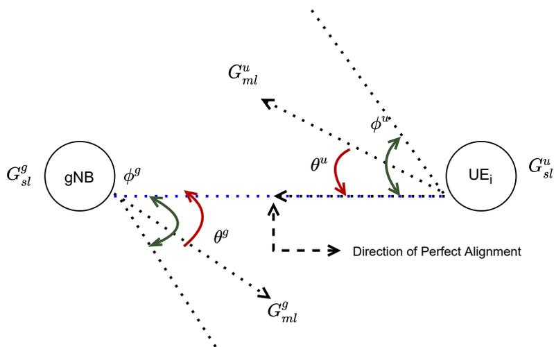
Figure 3.4: Antenna Model adapted from [18]. The figure depicts the alignment of gNB towards one of its users UE<sub>i</sub>. The misalignment of gNB towards its user is given by  $\theta$  and the gain of the main lobe is given by  $G_{ml}^{\phi^g}$ .
