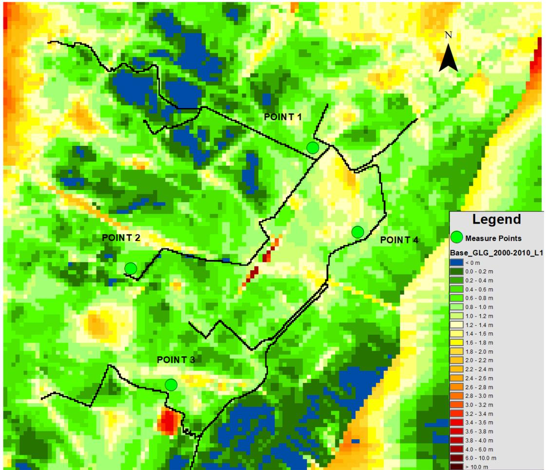
Figure 22: GLG results for the base scenario
