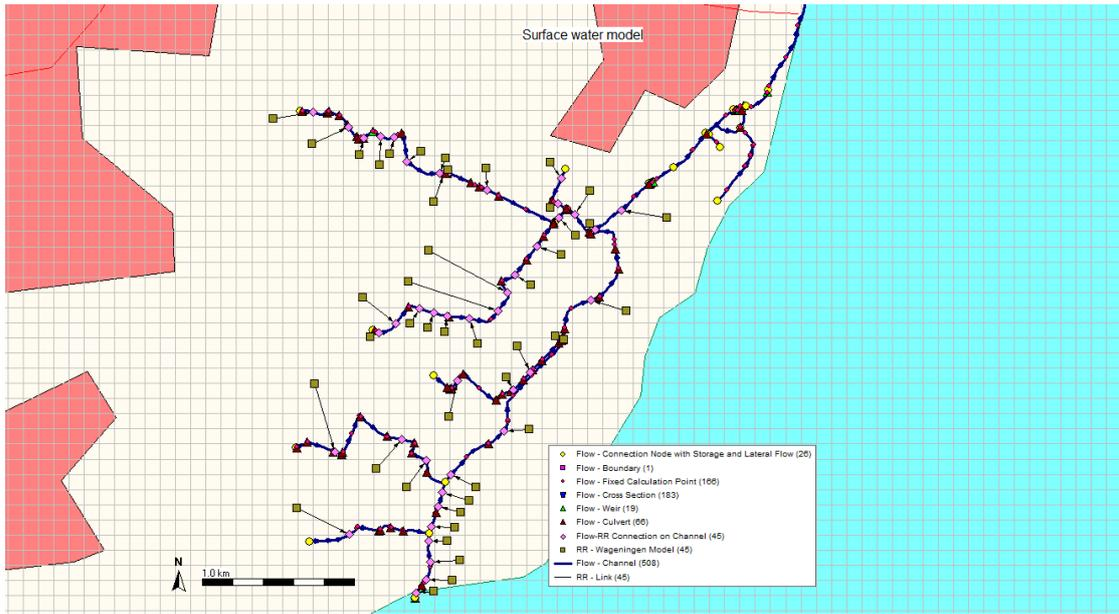
Figure 3: Surface water model network and nodes
