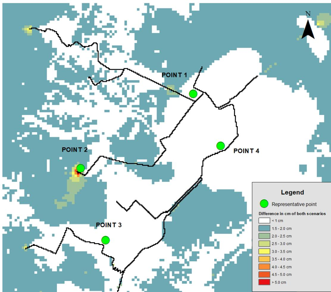
Figure 17: GLG map representing the effects of pinch culverts
