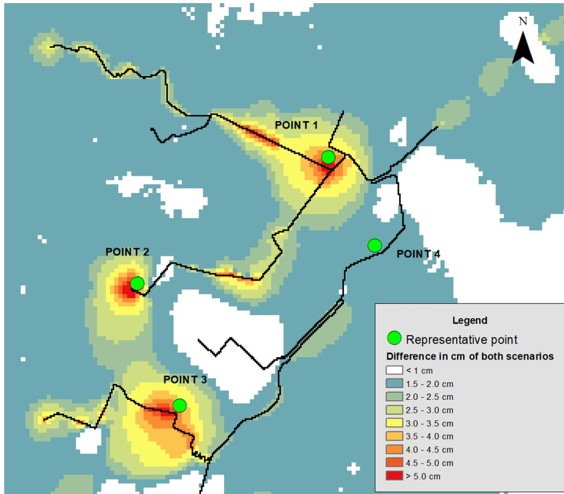
Figure 16: GHG map representing the effects of pinch culverts
