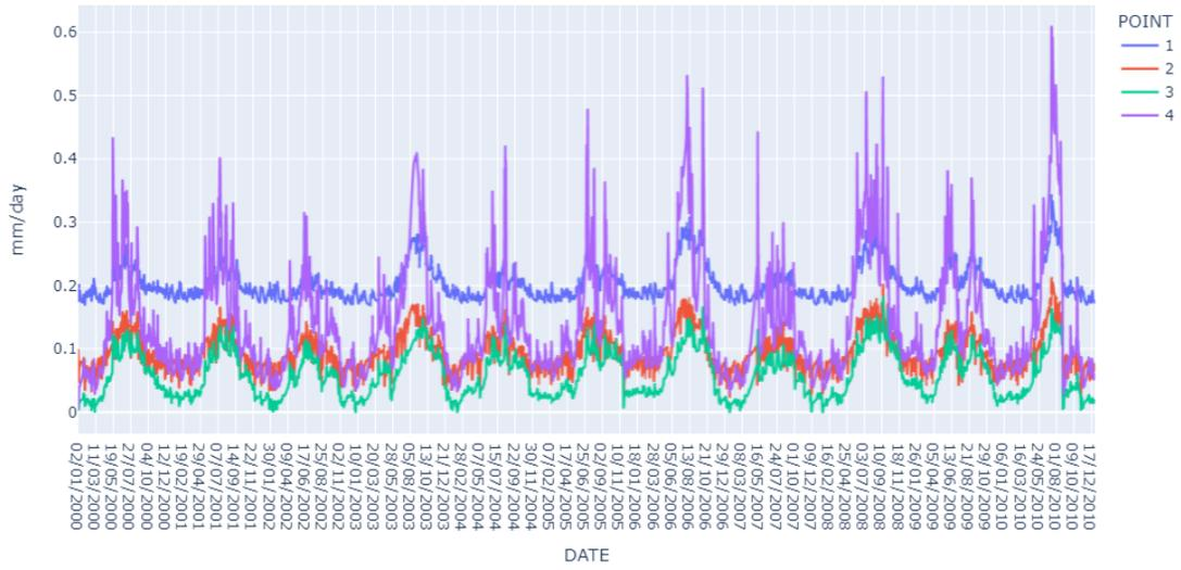
Figure 19: Infiltration values of the base scenario over a 10 year period
