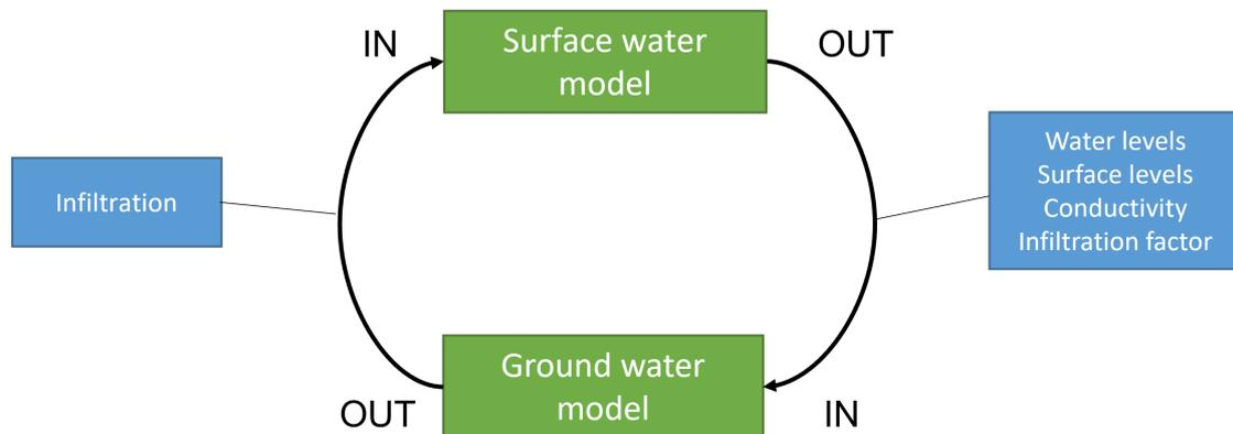
Figure 4: Diagram representing the interaction between the models
