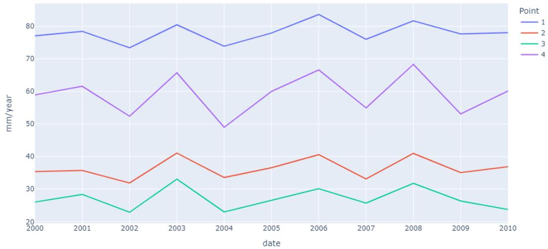
Figure 14: Infiltration results of the pinch culvert scenario over the ten years
