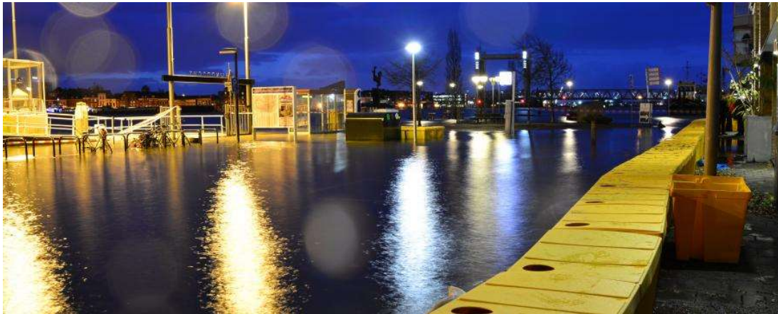
Figure 12 Box barrier (WaterWindow, 2021)
