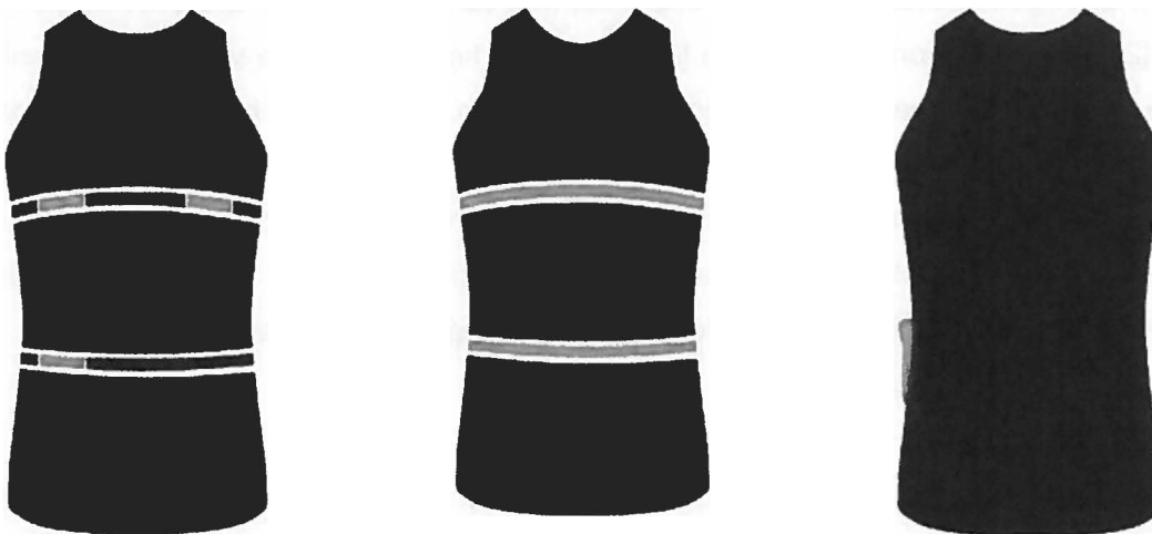
FIGURE 16: PLACEMENT OF (FROM LEFT TO RIGHT) ECG SENSORS, RIP SENSORS, AND 3-AXIAL ACCELEROMETERS
