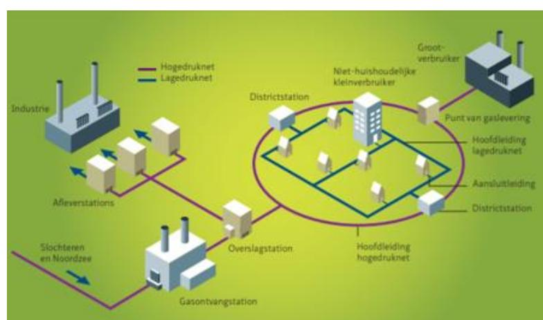
Figure 8: Example ring structure of gas network (Dutch) (Taselaar, 2009)
