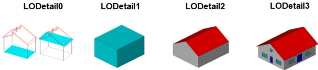
Figure 6: Implementation of CityGML's LODetail concept to a building (Kolbe et al., 2021)
