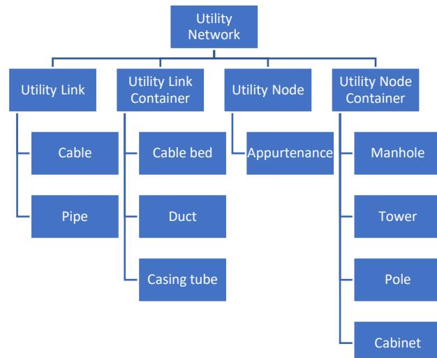
Figure 11: : Utility Network – Main elements as based on IMKL and INSPIRE
