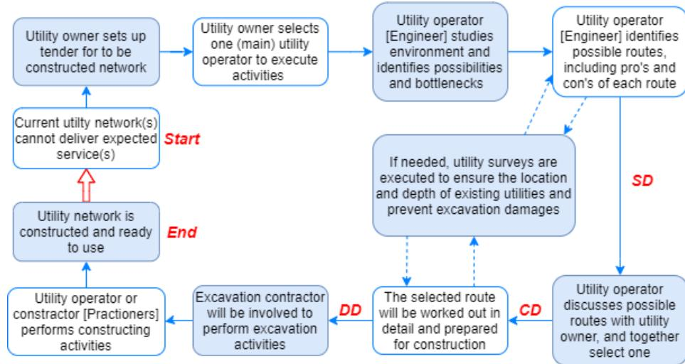
Figure 10: Generalized workflow design & construction of utility networks
