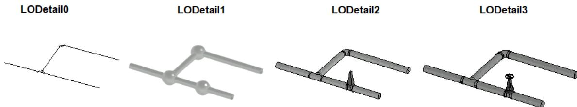
Figure 7: Geometrical representations of a segment of a Utility Network using an adapted LODetail framework (Becker et al., 2016; Kolbe et al., 2021)
