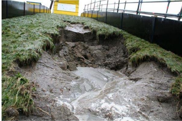
Figure 3 – An example of dike damage due to wave overtopping simulated by the wave overtopping simulator. Note: reprinted from Van der Meer et al. (2010).
