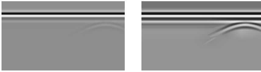
Figure 4.5: Before and After Contrast enhancement of Air void
