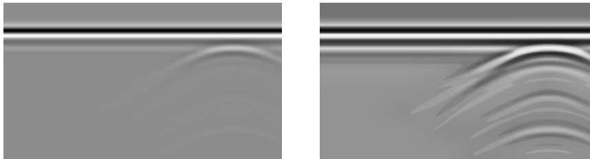
Figure 4.6: Before and After Contrast enhancement of Water void
