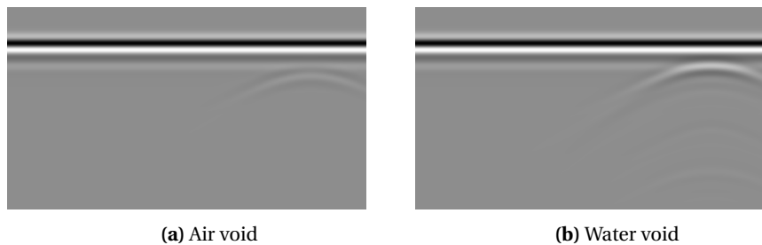
Figure 4.3: Radargrams of the corresponding environment as visualised in Figure 4.2
