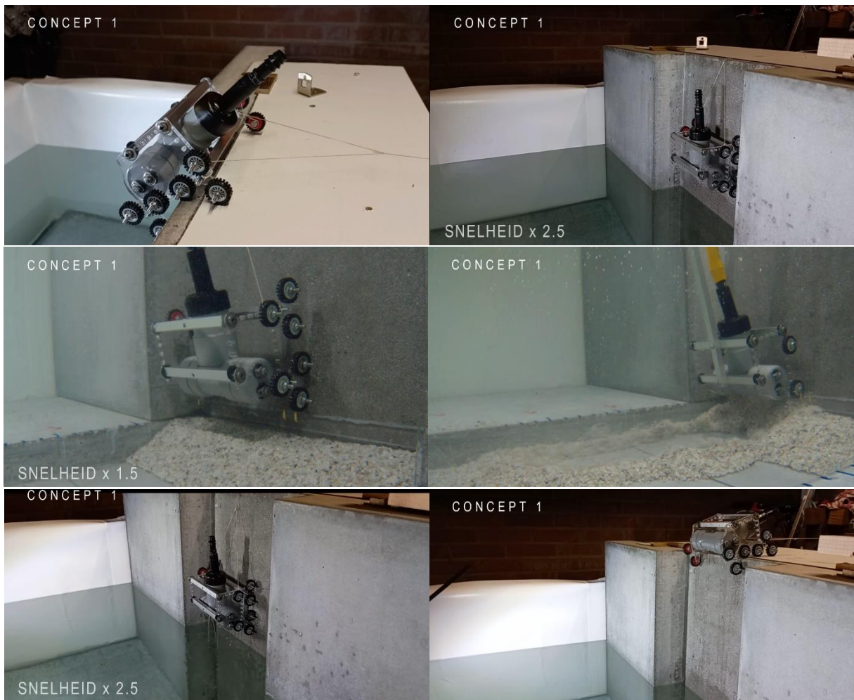
Figure 45. From left to right (per row) the cycle of concept 1: "walking" over the edge, lowering into the recess, lowering into place at the bottom, removal of siltation with the waterjets, raising of the concept and finally "walking" back up the edge.
