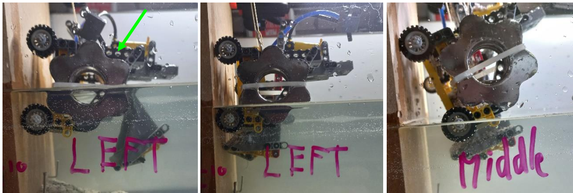
Figure 34. slanted with open scoop (left), stable with closed and filled scoop (middle), slanted with closed and filled scoop (right)
