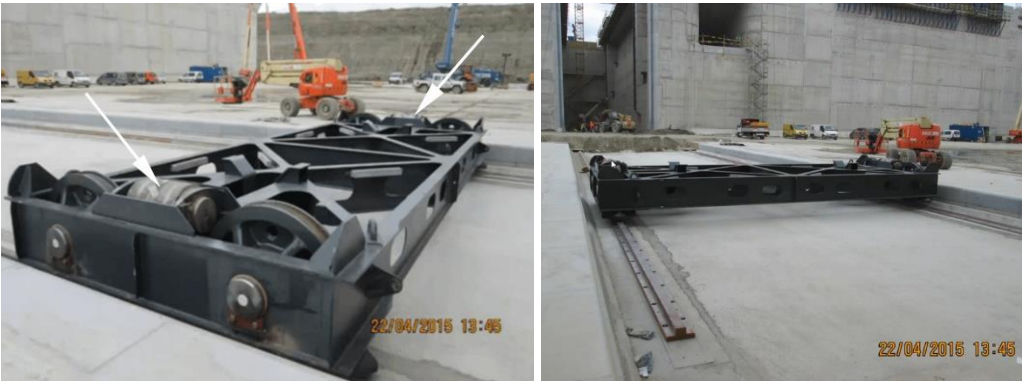
Figure 55. Undercarriage Kieldrecht lock [not to be copied without permission of Port of Antwerp].
