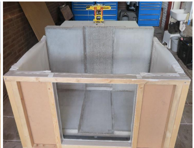
Figure 35. Concept 1 (top), Concept 2 (bottom left), concrete scale model of a gate recess within the water tank (bottom right).
