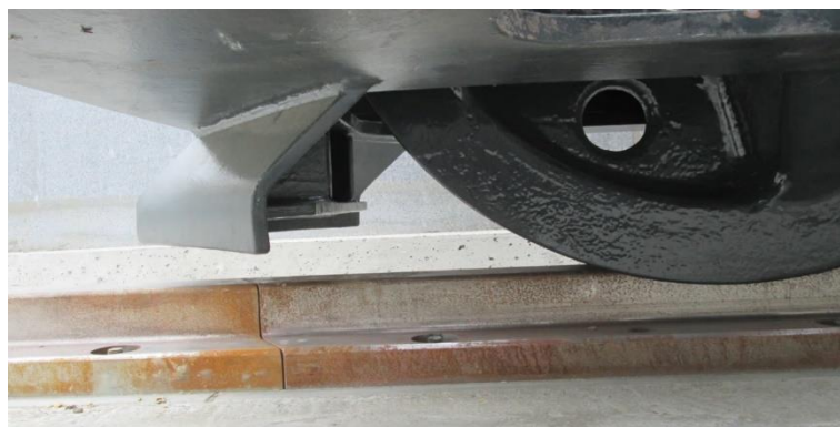
Figure 12. Plough in front of the wheels [23][not to be copied without permission of Port of Antwerp].
