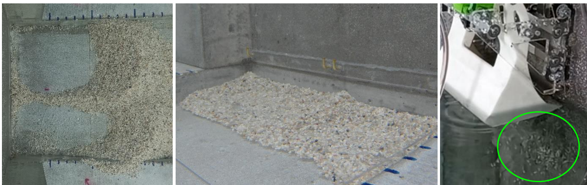
Figure 44. Concept 1 barrier slot 3 (left), concept 2 subsequent to six cleaning operations (middle), siltation falling out of the scoop encircled in green (right).
