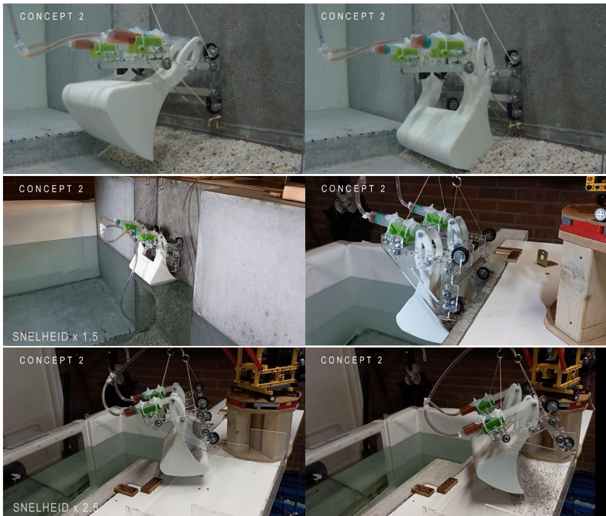
Figure 46. Note: the figure starts on the previous page. From left to right (per row) the cycle of concept 2: turning with the crane, lowering the concept over the edge, lowering into the recess (scoop closed), opening of the scoop before further lowering the concept, lowering onto the pins with the anchor points, removal of siltation with the scoop, raising the concept with a full scoop, raising the concept over the edge, turning with the crane and emptying of the scoop.
