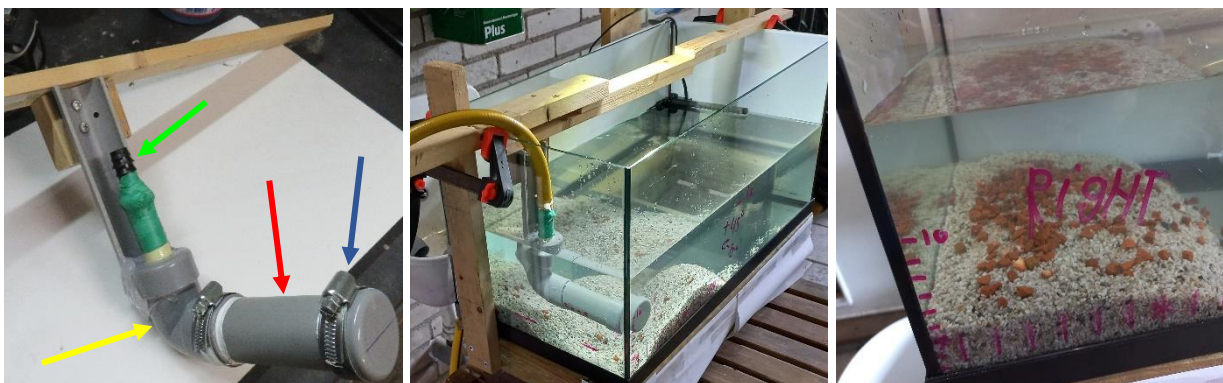
Figure 26. Prototype concept 1 (left), test set-up jet configuration (middle), aquarium with grid markings (right).
