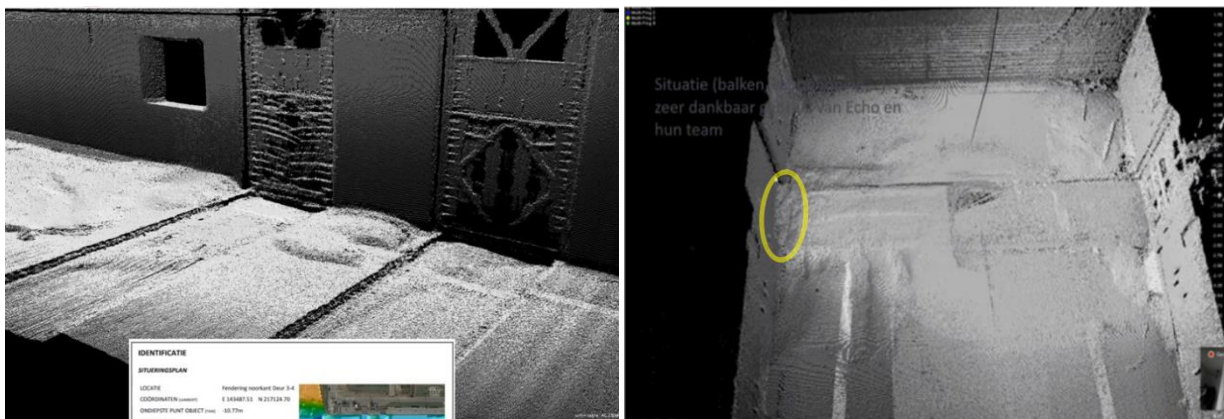
Figure 14. Echo picture of siltation in “non-problematic area’s” (left), echo picture of siltation of the gate recesses in Port of Antwerp (right) [24][not to be copied without permission of Port of Antwerp].
