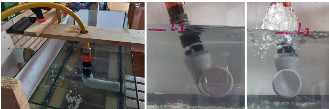
Figure 33. Stability set-up (left), slanted prototype (middle), upwards motion cancelled by upward jets (right).
