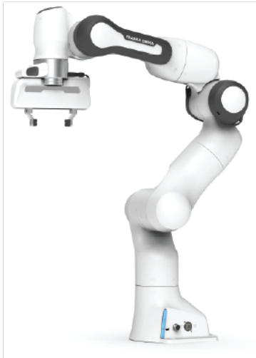
Figure 1.2: The Franka Emika Panda robot. It is a 7-DoF manipulator with a reach of 0.855 m and can carry a payload up to 3 kg. Besides that it is equipped with link-side torque sensors in each joint and an independently controllable gripper with a maximum width of 0.080 m.
