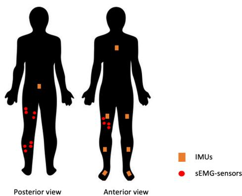
**Figure 2.1** Schematic representation of the subject' leg with the attached sEMG sensors in red and IMUs in orange. sEMG = surface electromyography, IMUs = inertial measurement units.
