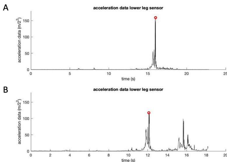
**Figure 2.2** Accelerometer data plotted for the sensor located on the lower leg. The circle indicates the peak used for detection of initial contact. A) acceleration data during a successful trial, B) acceleration data during failed trial.
