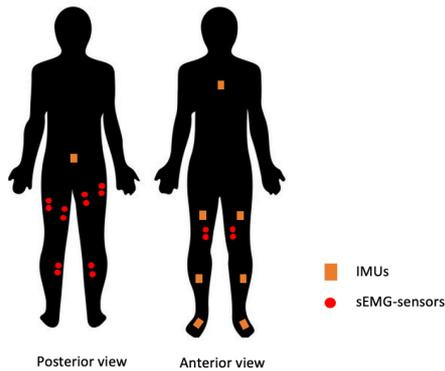
**Figure 3.1** Schematic representation of the participants' leg with the attached sEMG sensors in red and IMUs in orange
