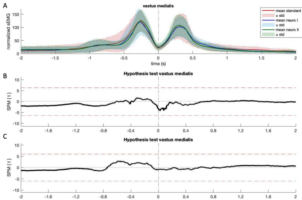
**Figure A2** A) Normalized sEMG values for the vastus medialis during standard SLHDs (red), the first neurocognitive SLHDs (blue) and the second neurocognitive SLHDs (green) in the control group. The solid lines reflect the mean sEMG, the shaded areas reflect the standard deviation. B) statistical parametric mapping outcomes for sEMG for standard SLHD and the first neurocognitive SLHDs C) statistical parametric mapping outcomes for sEMG for standard SLHD and the second neurocognitive SLHDs.
