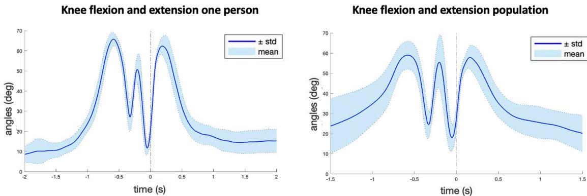
**Figure 2.5** Knee flexion and extension angles. A) mean of ten jumps for one person and B) mean of total population. The solid line reflects the mean, with the shaded area reflecting the standard deviation. Vertical line indicates IC.
