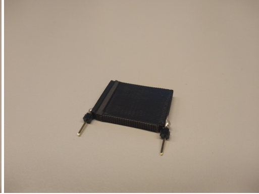
Figure F.6: Nine plates - Iron dielectric
