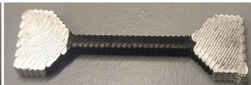
Figure E.10: 60 Degree - meander
