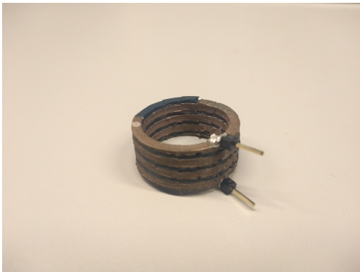
Figure F.7: Three windings - Air core
