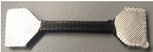
Figure E.7: 45 Degree - lines
