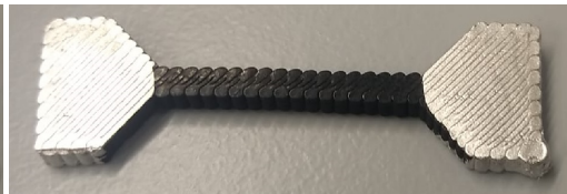
Figure E.8: 45 Degree - meander
