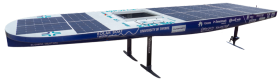
Figure 1. A picture of the vessel "Echo" of Solar Boat Twente, having 3 hydrofoils attached underneath. Photo by Solar Boat Twente.
