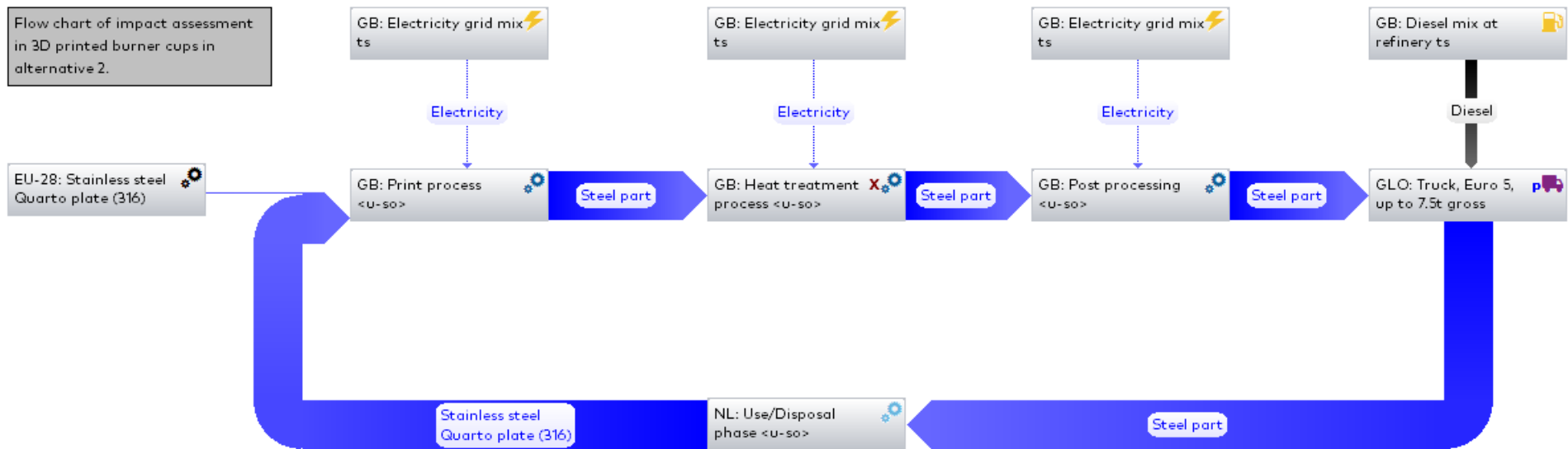
Figure 15: Flow chart of impact assessment in 3D printed burner cups in alternative 2: outsource + MOQ + AM.
