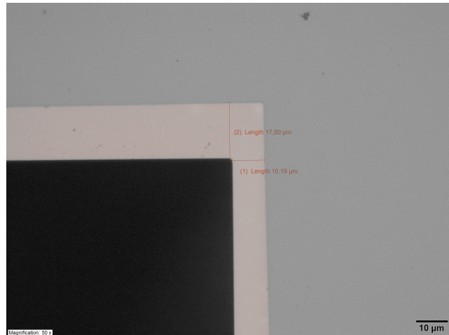
Figure 6.4: Undercut of the back mask. The misalignment angle, or the angle between the black square and light outlines, showed to be 0.5^\circ , the undercut from top to bottom measured 17.5 \mu\text{m} , the undercut from right to left measured 10 \mu\text{m} .
