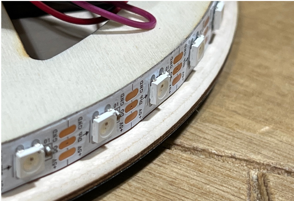
Figure 49 - Close-up of the LED-strip
