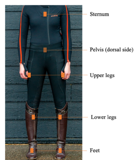
Figure 1: Sensor set-up of the MVN Link system with riding breeches and boots worn over the Lycra suit.
