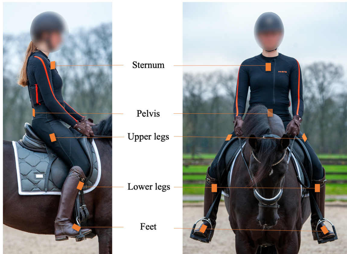
Figure 2: Sensor set-up of the MVN Link system with riding breeches and boots worn over the suit, as the participant is sitting on the horse.
