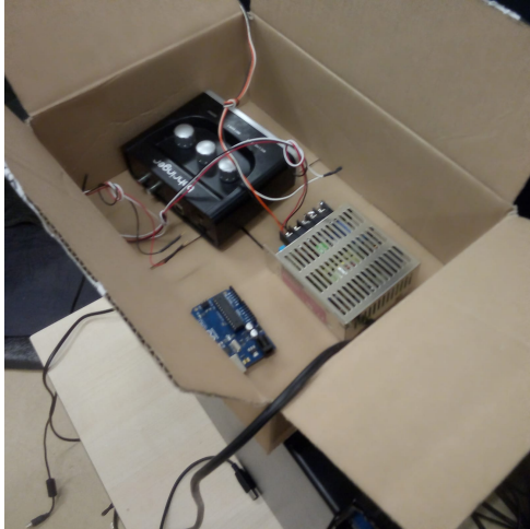
(a) An Arduino Uno, an external power supply and an Audio interface
