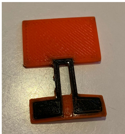
Figure A.1: Short circuited 3D printed flow sensor
