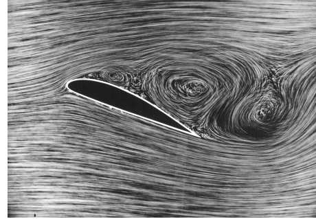
Figure 2.4: Flow separation around an airfoil (Wikipedia contributors, 2021b)
