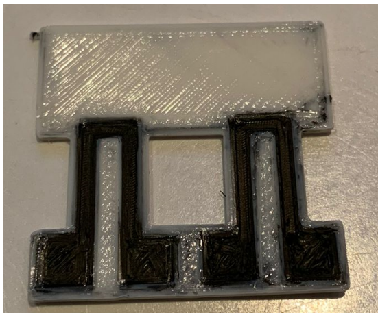
Figure A.2: Sensor with four strain gauges
