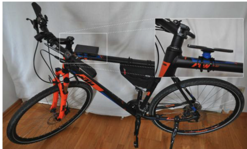
Figure 5.23: Measuring accelerations with smartphone for road roughness analysis [59]
