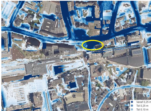
Figure 4: Water depth 't Bólke at precipitation event of 70 mm in one hour. Source: (Twents Waternet, 2015).
