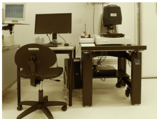
Figure C.2 White light interferometry in NanoLab
