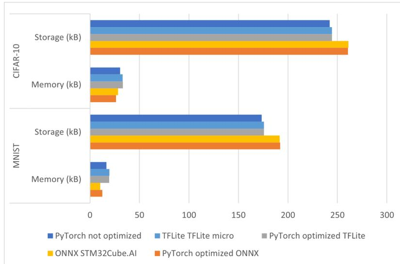
Figure 5.1: Memory and storage predictions from the NAS algorithm (blue), plotted with the STM32Cube.AI analysis results (grey, yellow) and overhead-optimized predictions (light blue, orange)
