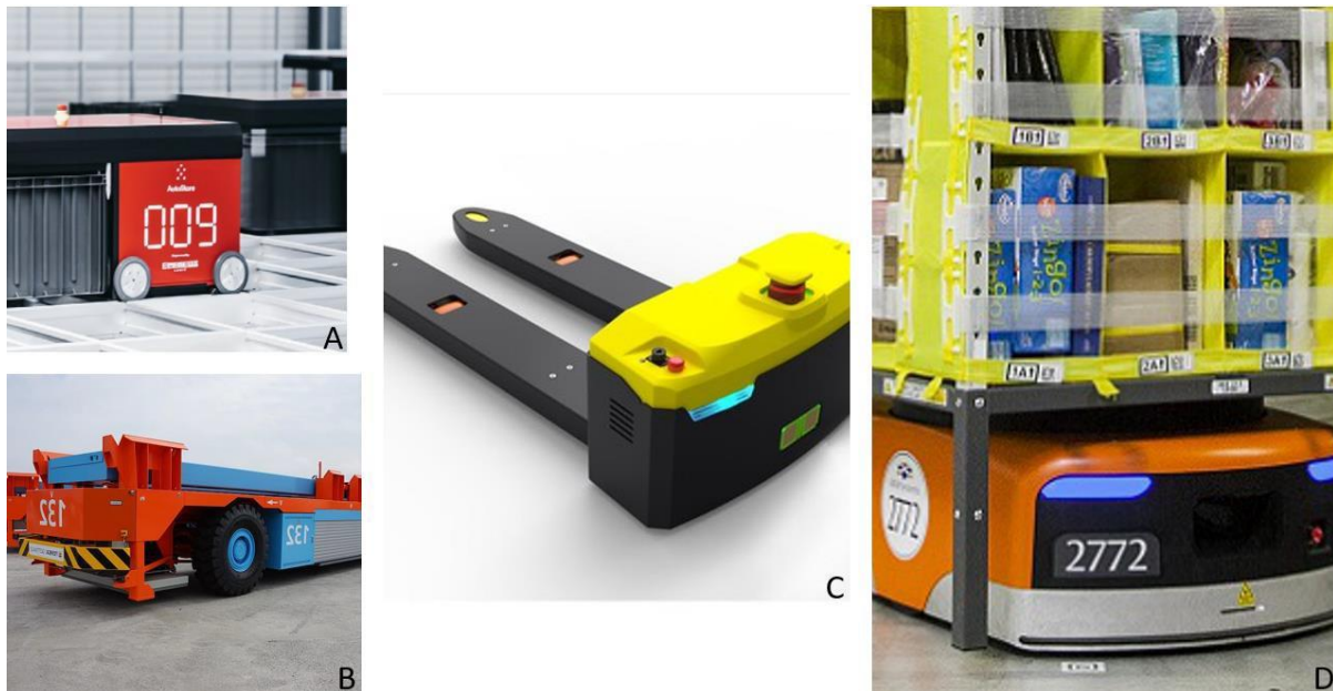
Additional information: A = AGV used by Autostore; B = AGV that is used for the transport of containers in the port of Rotterdam; C = AGV that is often used for movements within a warehouse; D = AGV that moves stock cabinets and is used by Amazon.
