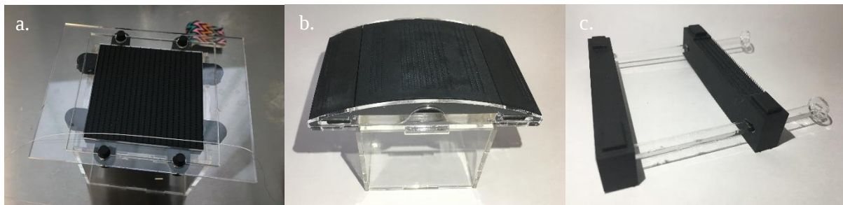
Figure 4-10: Prototypes a) Layered mould, b) Segmented mould, and c) Stretch mould.
