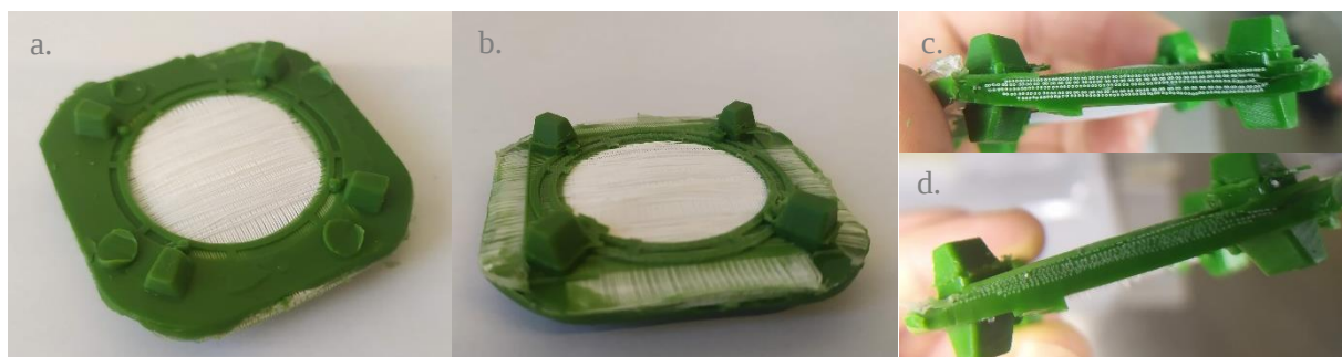
Figure 5-3: A potted combined oxygenation and hemofiltration fibre membrane bundle. Uncut top view (a) and bottom view (b). After cutting the oxygenation fibres (c) and hemofiltration fibres (d) were open on visual inspection.
