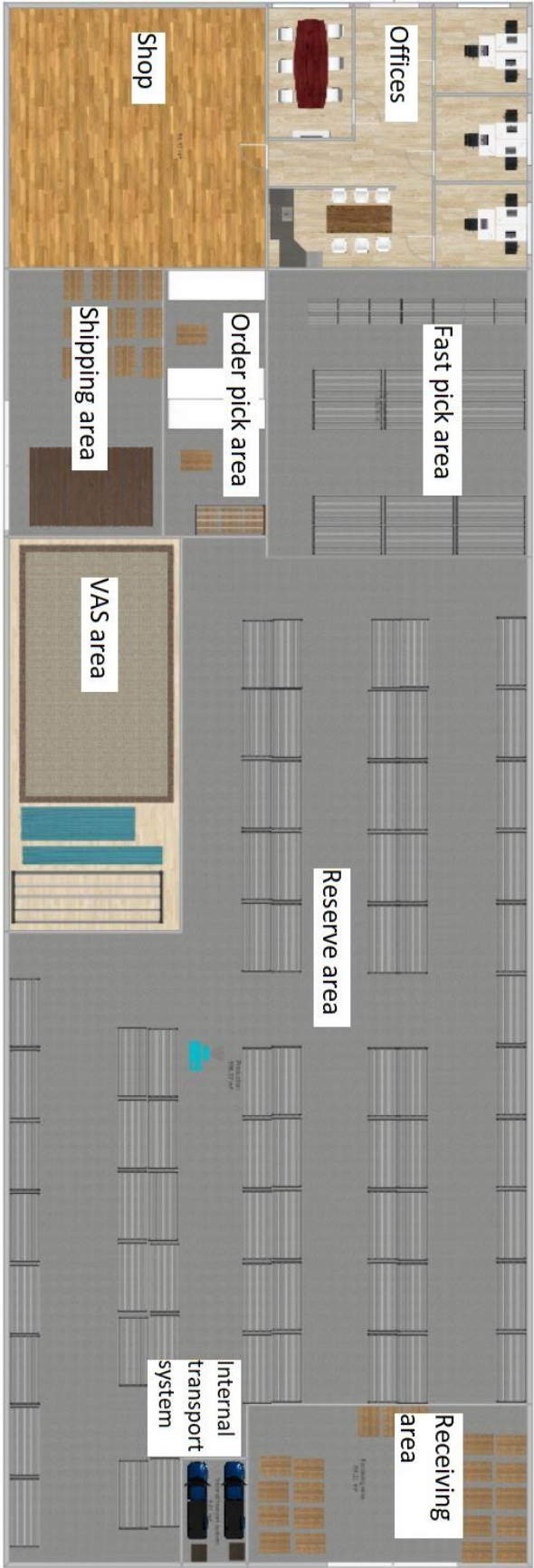
Figure 42 - Final warehouse layout
