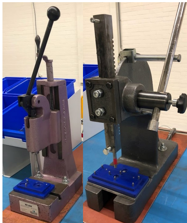
Figure 8.2: Difference between manual press types: left press with adjustable working height, fixed outreach, and spring-loaded handle and the right press having none of these features.
