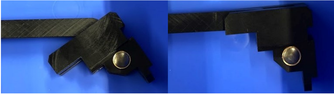
Figure 8.1: Difference in resistance between glued (r) and unglued bush bearings (l) causing the pivot block to tip forward (l) or not (r).
