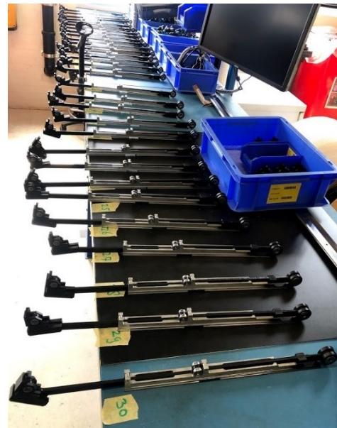
Figure 3.3: Lever arrangement for the attribute agreement analysis.
