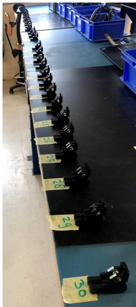
Figure 3.2: Pivot block arrangement for the attribute agreement analysis.
