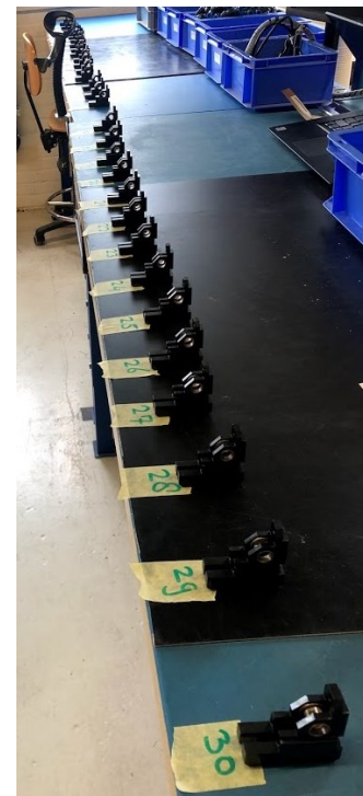
Figure H.1: Pivot block arrangement for the attribute agreement analysis.
