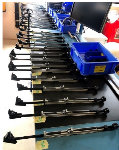
Figure H.3: Lever arrangement for the attribute agreement analysis.
