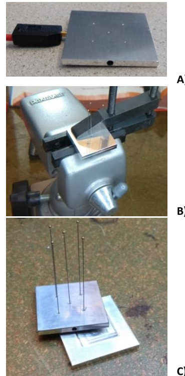
Figure 3.9 Assembly of the needles into the base plate
