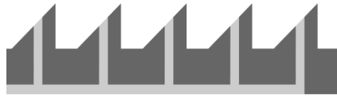
Figure 3.3 The etched hollow microneedle design. Dark grey is the silicon wafer, and light grey is the electrical conductive material.
