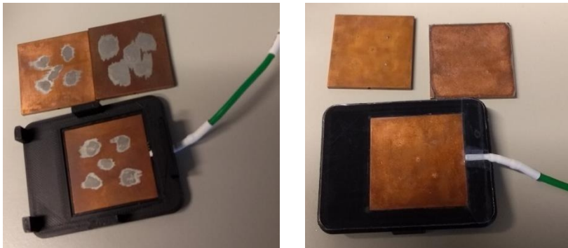
Figure A.2 A) shows the oxidation of the ThESSA electrode after several weeks. The heating of the copper increased the oxidation. The upper right electrode and the one in the holder were used in combination with the thermode, whereas the upper left was not (it was earlier on disqualified, and therefore not used). B) The top of the electrode is less oxidized due to the covering tape.
