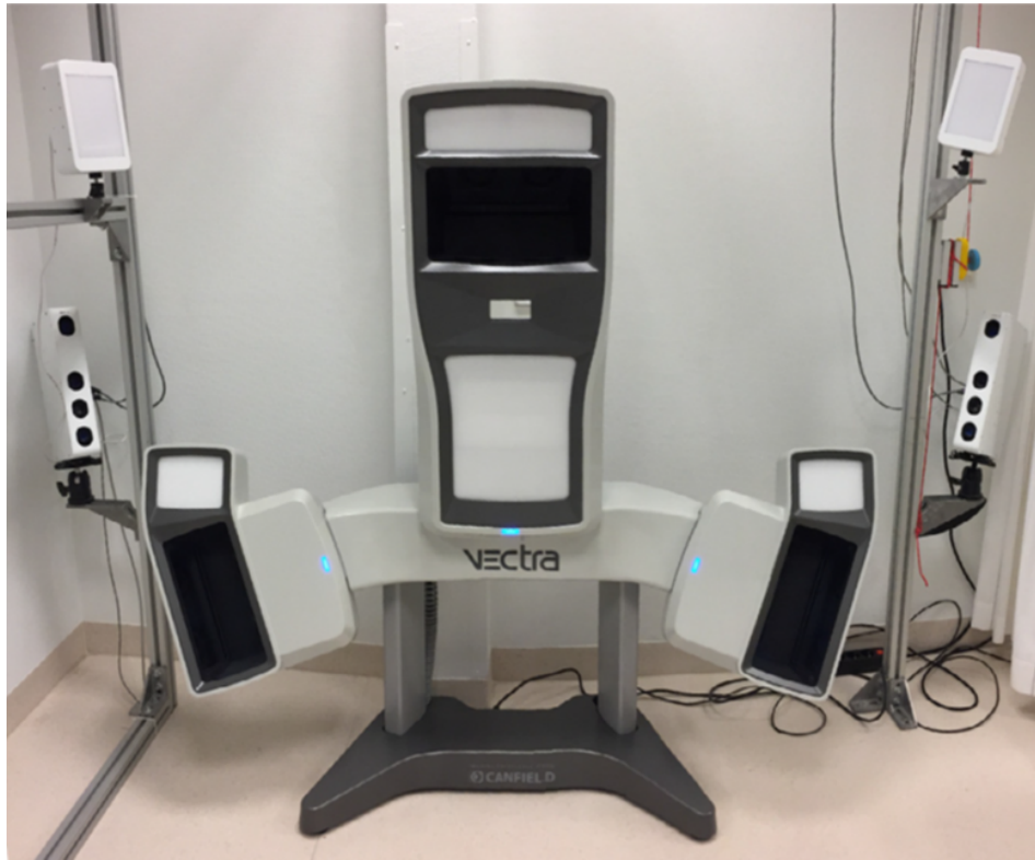
Figure B.2: A photo of the passive Canfield Vectra XT system and the hybrid 3DMD system around the Vectra
