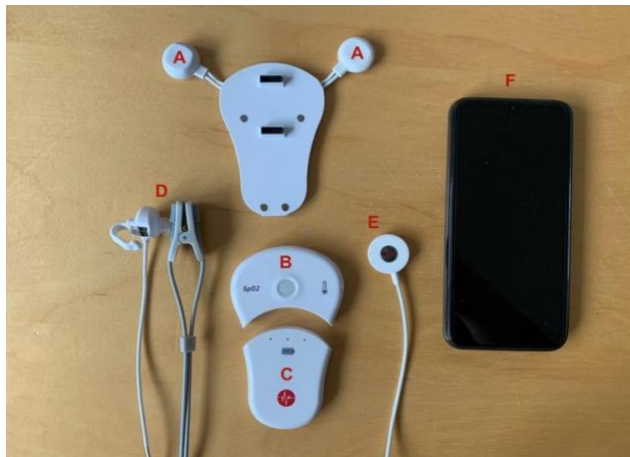
Figure 1: The Nightingale sensor, with the ECG module (A), SpO2 and temperature module (B), rechargeable battery (C), ear sensors (D), temperature sensor (E) and relay device (F).
