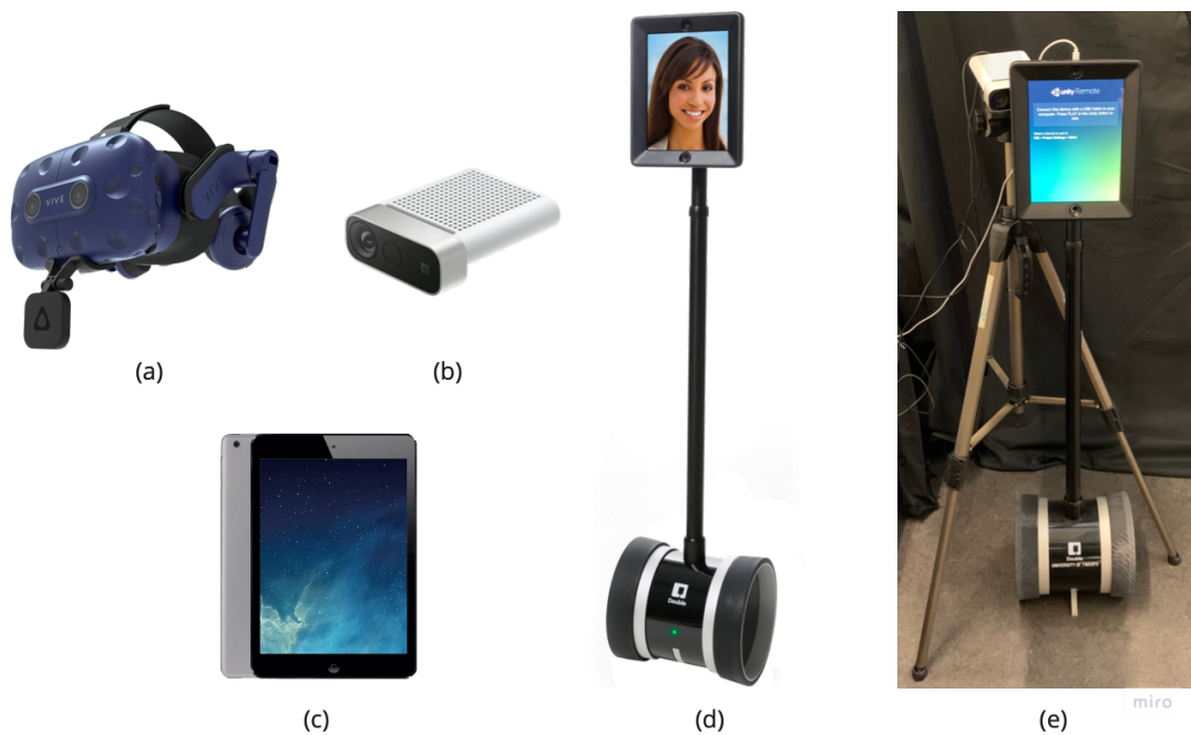
Figure 3.7: Hardware used: (a) HTC VIVE Pro Eye with Facial Tracker attached. (b) Microsoft Azure Kinect DK for live video capture. (c) iPad Air 1st Generation to display avatars as an Unity Remote output. (d) Double 2 telepresence robot with iPad mounted. (e) Our setup to display avatar of the user wearing VR HMD along with Kinect camera for video capture of the interactant.
