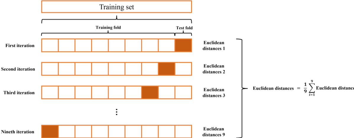
Fig. 8. Illustration of the nine-fold cross-validation for evaluation of the renal artery ostia detection network’s performance.
