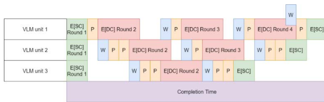
Figure 32: Illustration of completion time for the example order with multiple VLM units
