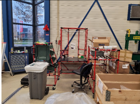
Pipe and joint worktable
