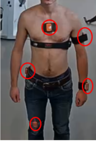
Figure 2. Photo of the Zephyr BioHarness and five Xsens IMUs (circled in red) as worn during the experiment. The resolution of this figure is low, as it was taken from a video recording. This participant is left-handed.
