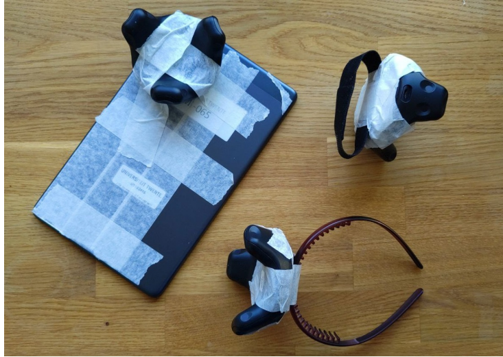
Figure 33: Picture of the three IVR trackers used in the second iteration evaluation, attached to a tablet, hairband, and velcro hand strap.
