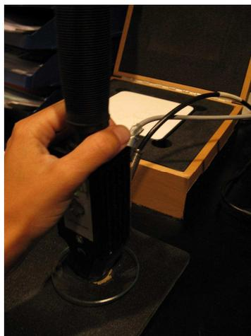
*Figure 2-3: Photo illustrating the procedure in taking spectral measurements. The light emitted from the contact probe is reflected from the target and measured from the instrument.*
