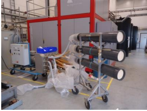
Figure 15: Modules attached to the drying machine
