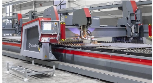
Figure 1.2: V310 plasma cutting and drilling machine, including the Cutting Tables (Voortman Steel Machinery, 2021).
