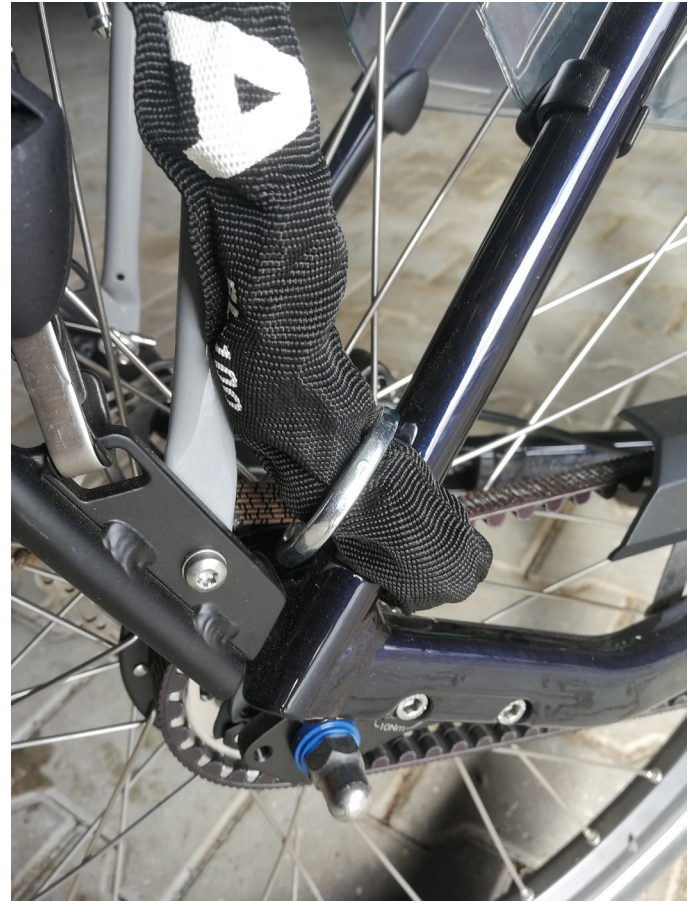
Figure 67: Example of how the chain will be mounted to the frame by looping it around the seat stay
