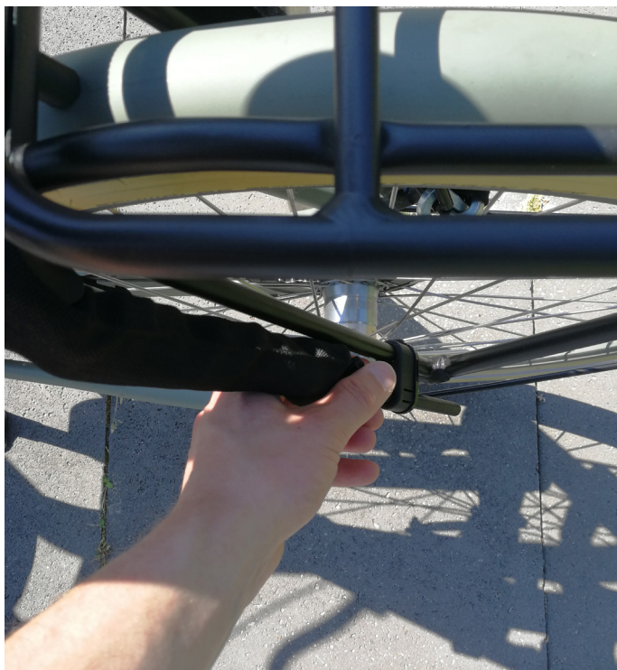
Figure 108: Take the lock pin out of the holder.
