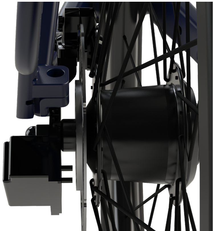
Figure 58: Rear view of the brake disc lock. As can be seen there are two lock pins and there is still clearance between the slotted disc and the dropout pad.
