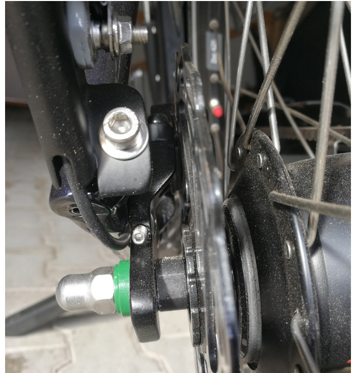
Figure 47: Dropout pad to brake disc clearance
