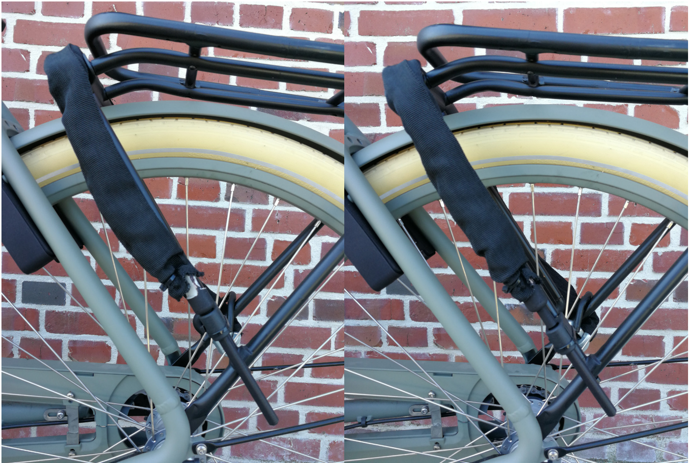
Figure 103: As can be seen in this picture, the lock pin is fully inserted in the lock pin holder while still having some slack left in the chain.
