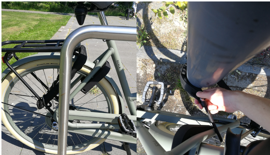
Figure 106: Line up the bike with the pole between the chain loop and the locking mechanism. Figure 107: Parking the hole in front of the pole will make it harder to insert the long lock pin.
