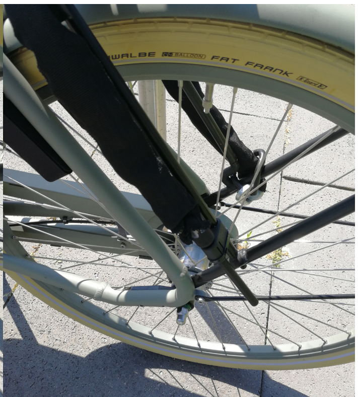
Figure 116: When the chain has been correctly guided around the carrier it can be fully inserted into the holder.
