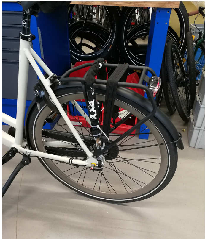
Figure 68: Test setup to test whether the chain will slap around during cycling.
