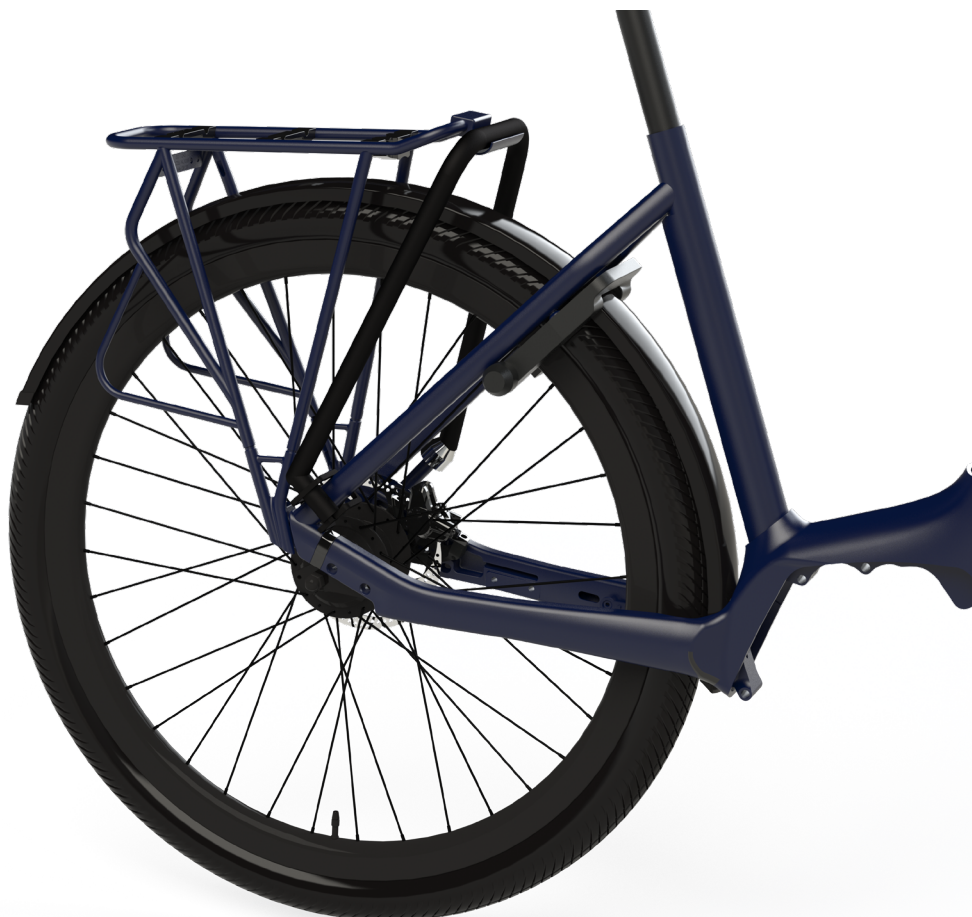
Figure 71: Right side render of the integrated chain lock concept with the chain holder, the chain looped around the frame and the lock itself.
