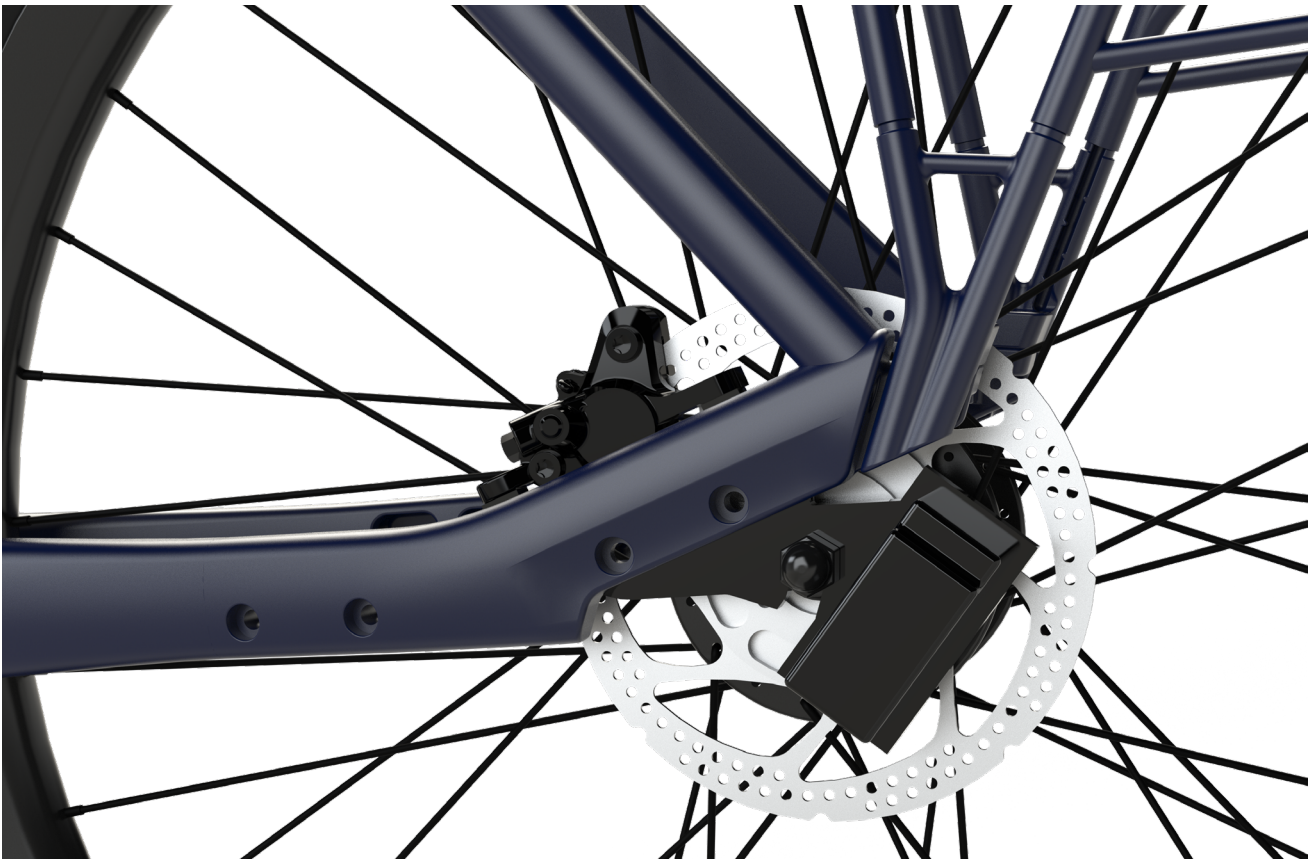
Figure 57: Close up of the brake disc lock. As can be seen, the wheelaxle can still be removed from the dropout pad without touching the solenoid box.
