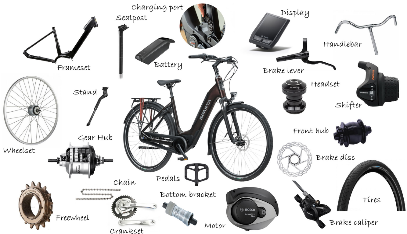
Figure 17: overview of bicycle components that can be used for locking a bicycle.
