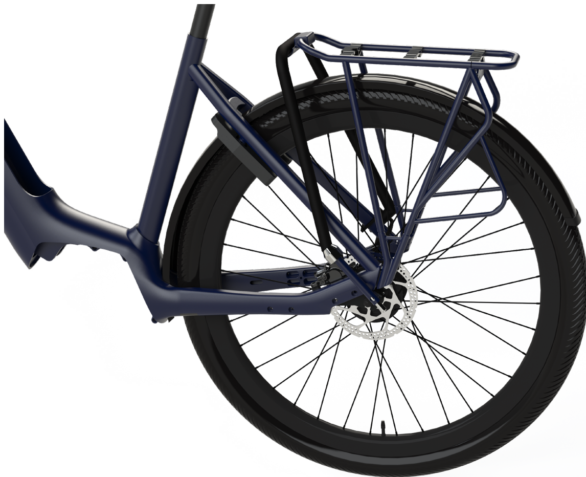
Figure 70: Left side render of the integrated chain lock concept with the chain holder, the pin holder and the lock itself.
