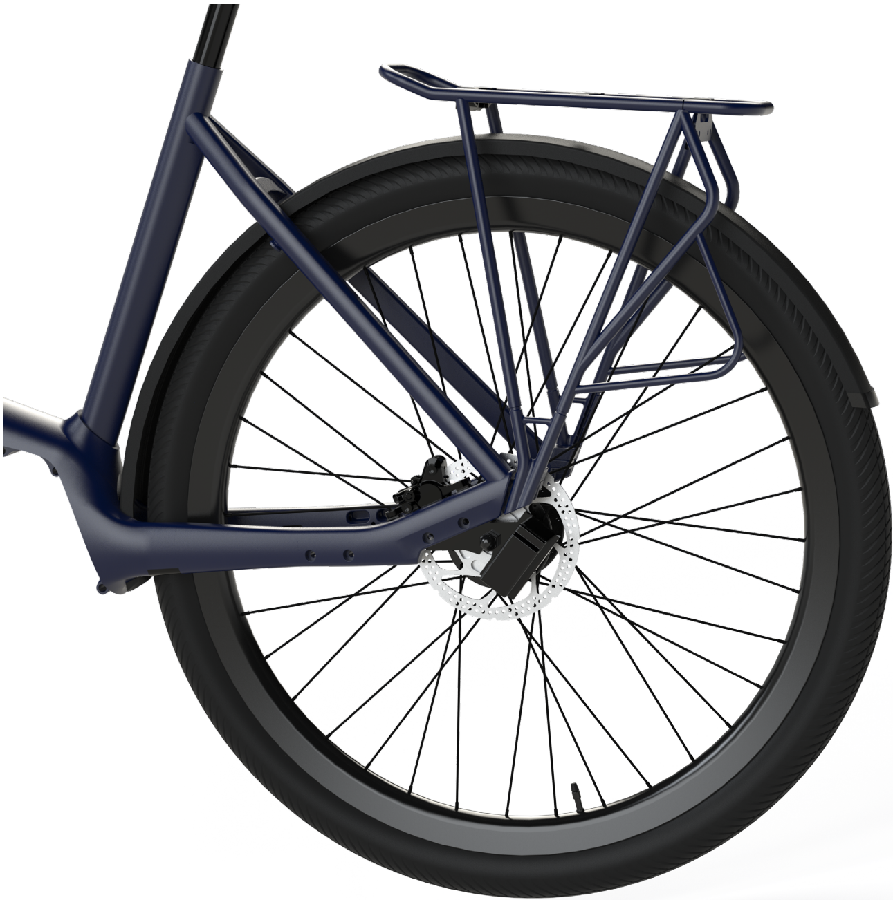
Figure 56: This render shows the brake disc lock concept with the solenoid box integrated in the dropout pad and the slotted disc in front of the brake disc.
