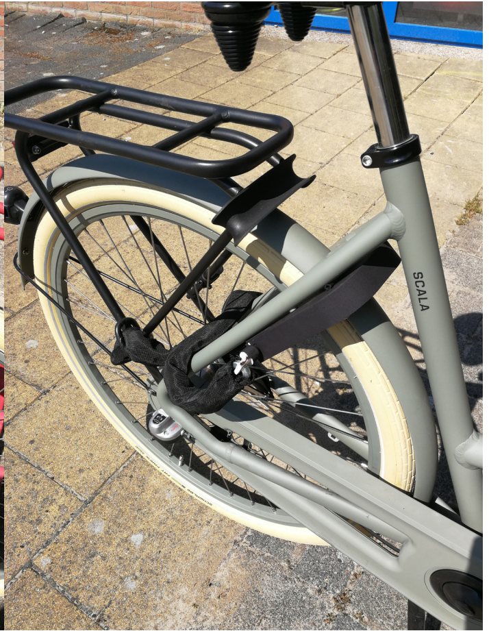
Figure 100: This lock can not reach the rack, but it can be looped through the rear wheel.
