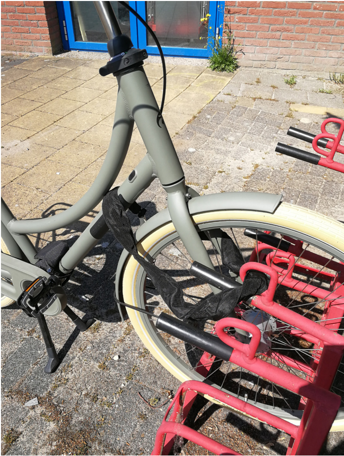
Figure 99: A regular chain lock can lock the frontwheel to the bike rack.
