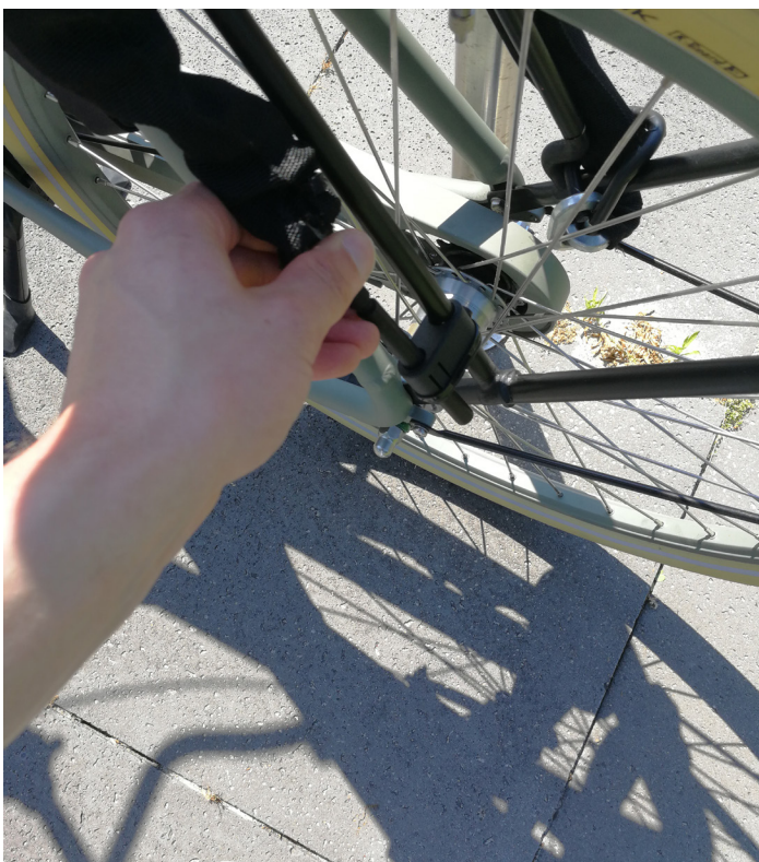
Figure 115: Put the lock pin in the lock pin holder.
