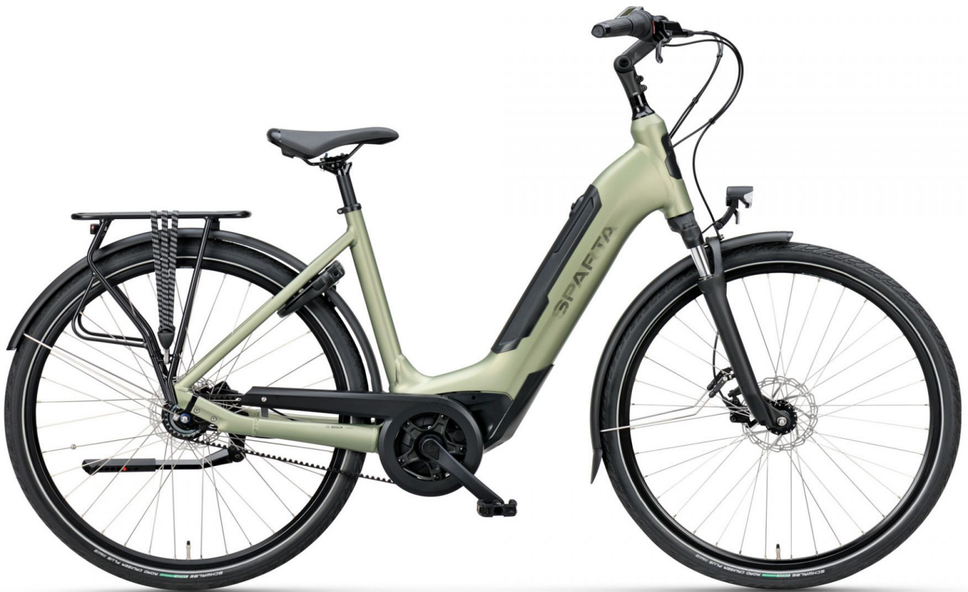
Figure 5: The Sparta C-GRID ULTRA, an e-bike that is according the latest trends: mid engine from Bosch; an in-tube battery; using a belt drive instead of a chain; having a low step through frame; using hydraulic disc brakes; and using an internal gear hub (Sparta, n.d.).
