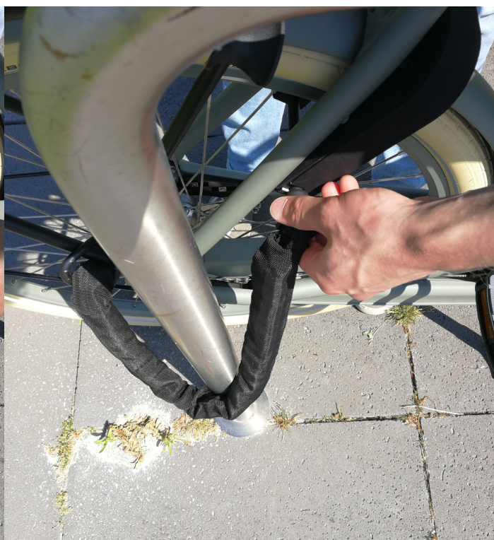
Figure 111: Push the lock pin all the way in. Then the lock will be locked.
