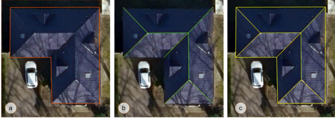
Figure 2. a) Building outlines; b) Inner rooflines ; c) Building roof structure
