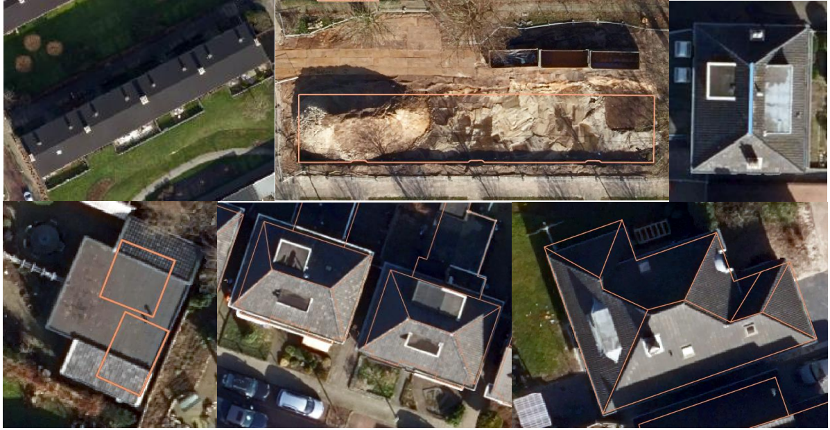
Figure 6. Mismatches of the reference data with 0.08 m resolution RGB image
