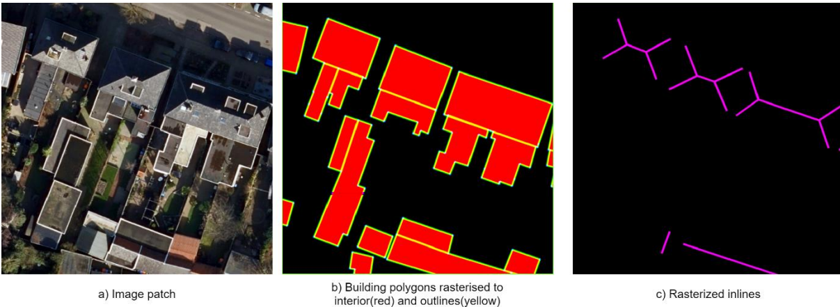
Figure 8. Pre-processing: rasterization of the reference data
