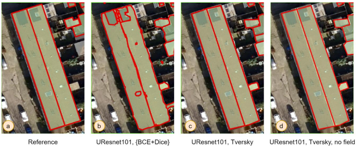
Figure 21. Rooflines of the building extracted by the models with {BCE+Dice} and Tversky losses. UResNet with {BCE+Dice} : PoLiS outline - 1.87 m, PoLiS inner roofline - 4.2 m; UResNet101 with Tversky : PoLiS outline - 0.16 m, PoLiS inner roofline - 0.05 m; UResNet101 with Tversky, no field : PoLiS outline - 0.13 m, PoLiS inner roofline - 0.17 m
