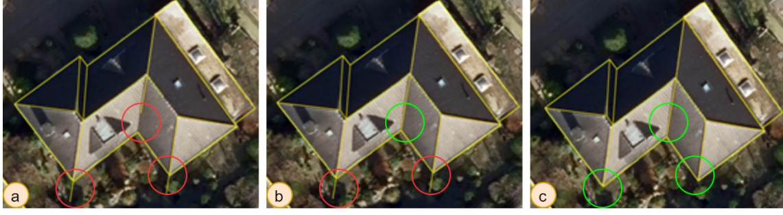
Figure 16. Post-processing: a) raw predicted output; b) post-line extension output; c) post-line trimming output
