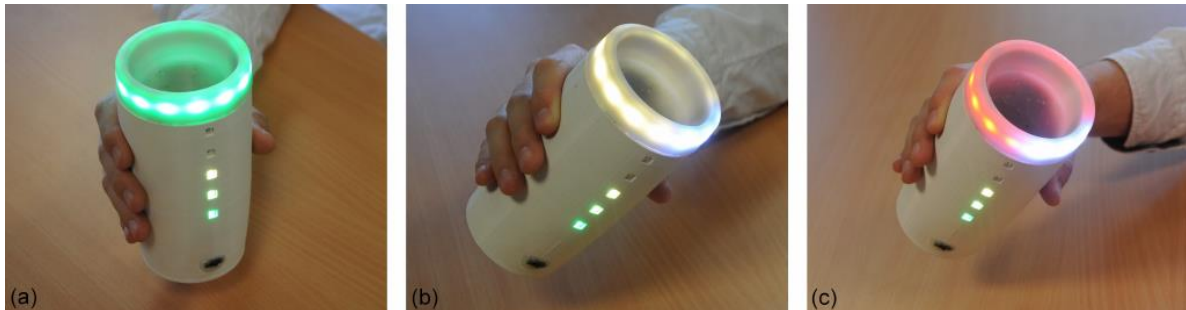
Figure 10. SyMPATHy prototype with LEDs on the side indicating the liquid level and LEDs on the top indicating the orientation: a) glass held vertically (0-20°); b) glass tilted somewhat (20-50°); c) glass tilted (>50°). The figure is taken from [24].
