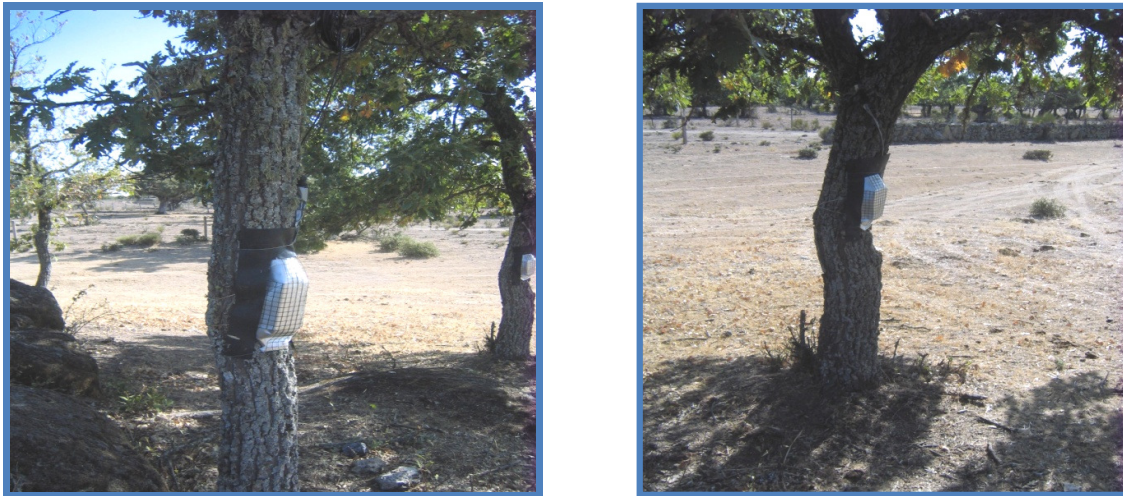
Figure 4-4: Set up of Sun Shielded Granier TDP Q. pyrenaica Trees - Trabadillo 2009
